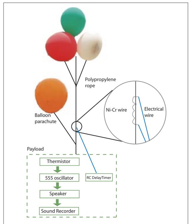
**Fig. 1. Schematic diagram of the sounding balloon experiment.**
