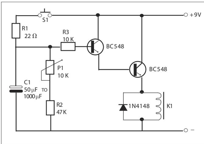
**Fig. 2.** Diagram of timer circuit used to liberate balloon parachute and its payload. The contacts (not shown) of relay K1 switch on power to Ni-Cr wire.
