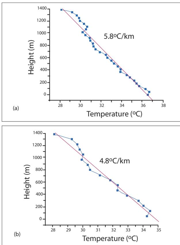
**Fig. 6. Temperature profiles during (a) ascension and (b) the fall.**
