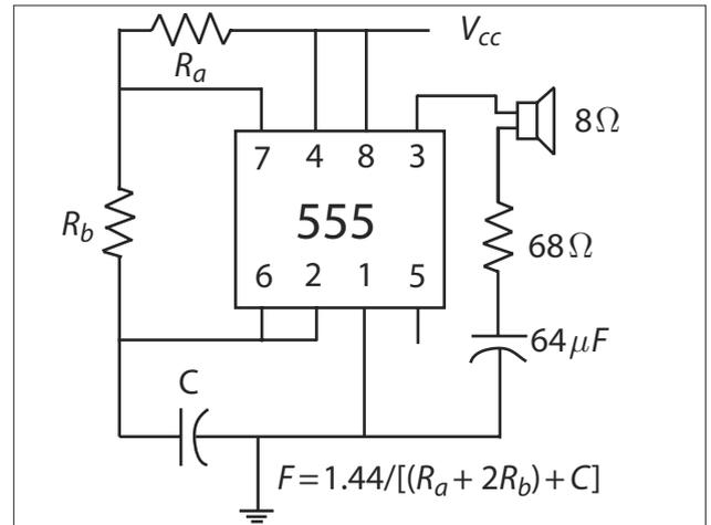
**Fig. 3.** The oscillator circuit.  $F$  is the output sound frequency value.  $R_b$  is the NTC 10-k $\Omega$  thermistor. The values used for other components were:  $R_a = 2200 \Omega$ ,  $C = 20 \text{ nF}$ .
